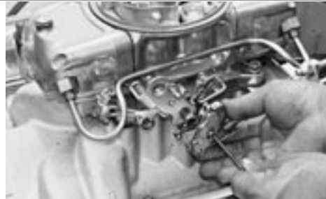
Next, install the TV cable and the cam adjuster cap. The cap will hold the cable and adjustment screw in place. Reinstall the accelerator cable as well.
