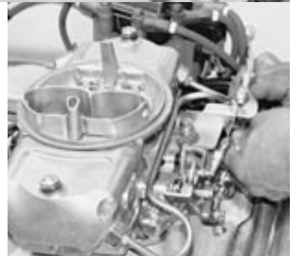
adjust the slack out of the accelerator cable before moving on. If the accelerator cable is adjusted perfectly, start the setup by pushing the "D"-shaped button while pushing the cable slider (the round piece of plastic attached to the cable) back towards the transmission until it stops as far into the cable housing as it will go. Release the "D" button to hold the cable in this pre-set position.
